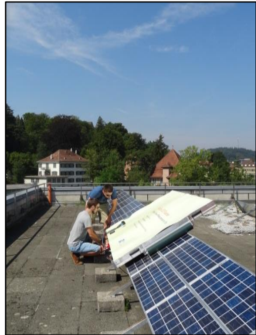
Use of the portable LED flasher on a flat roof
