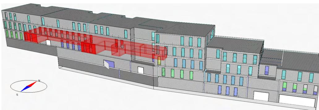
Fig. 1: IDA ICE simulation results. The heat demand is color-coded in the windows. A corridor zone is highlighted in red.
