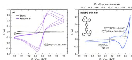
Fig. 2: Voltammograms of blank ITO and ITO/ferrocene (panel a) and of the ITO/PEDOT:PSS/NPB thin film (panel b).
