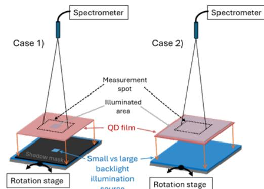
Fig. 2: Measurement setups to analyze the influence of the illumination geometry on the light conversion efficiency.
