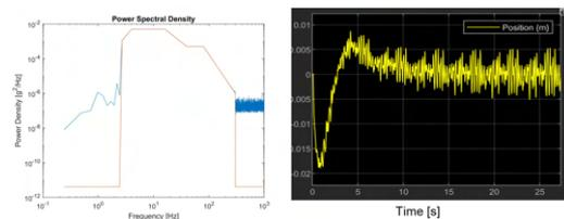
Fig. 3: Implementation of pre-control using gravity estimation. The left graph shows the target profile in red and the actual profile at  $T = 30s$  in blue. The graph on the right shows the initial outward movement, which has been significantly reduced and is within the position criteria.
