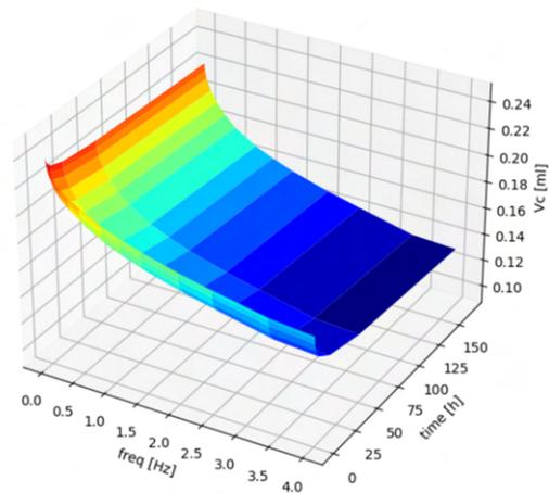
Fig. 2: Simulation results of the decreasing pump performance for a specific tube. It shows how the conveyed volume per cycle  $V_c$  decreases with higher pump frequencies (viscoelastic behavior) and over time (fatigue effect).
