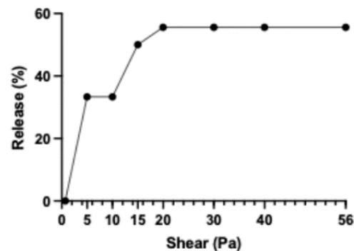
Fig. 2: Characteristic release curve of an HSL product. A pronounced increase in release is observed above a certain shear force.
