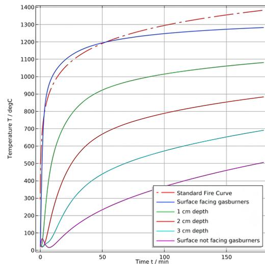
Fig. 2: Temperature profiles of the component being tested. The surface temperature of the component corresponds with satisfactory accuracy to the temperature profile prescribed by the regulatory bodies.
