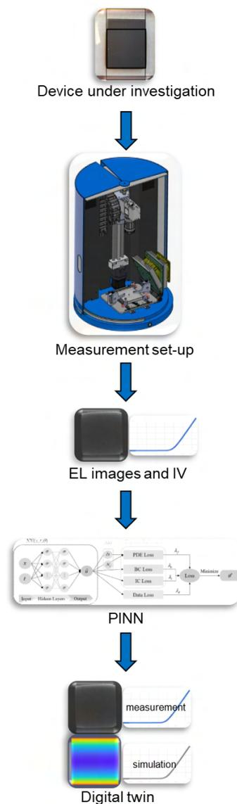
Fig. 1: Workflow for the generation of the digital twin
