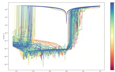
Fig. 1: Current-voltage curve of a resistive switch fabricated in our labs.
