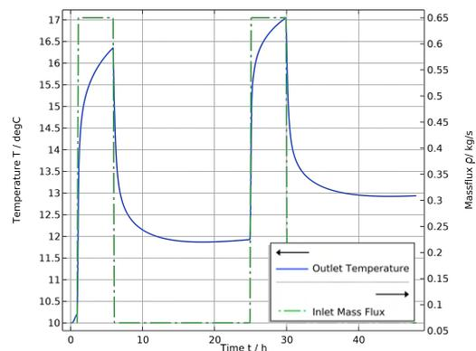
Fig. 2: Temperature at the outlet and mass flux at the inlet. Energy storage capabilities are shown in the offset of the two response peaks in the y-direction.
