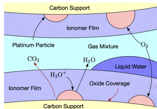
Fig. 1: Simplified model geometry of a mesopore in the CCL.
