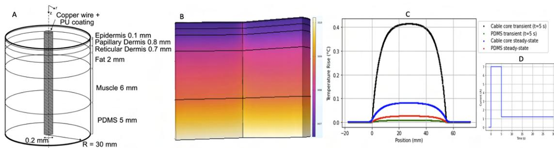
Fig. 1: A) Graphical representation of the 2D axisymmetric skin multilayered model [2]. B) Thermal distribution in COMSOL Multiphysics. Units: degrees Kelvin. C) Temperature rise in the core of the copper wire and in the PDMS due to inrush current and in the steady-state. D) Electrical conditions of the model.
