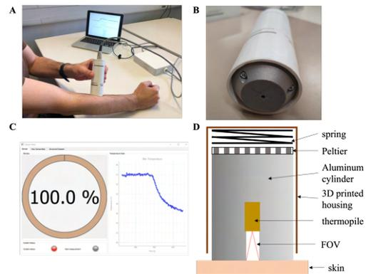
Fig. 1: A) Image of the device. B) Zoomed image of the hand-held device to illustrate the measuring opening of the device. C) User interface of the software. D) Diagram of the thermopile for measuring the transient temperature, which is installed in the hollow Peltier metal cylinder of the hand-held device.
