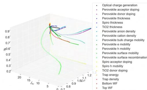
Fig. 1: 3D  $V_{oc} - J_{sc} - ff$  plot of the different parameters
