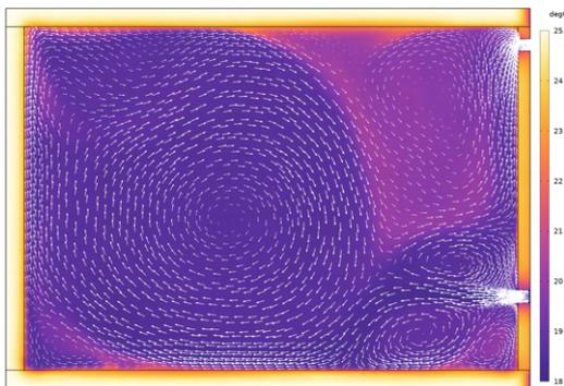
Fig. 1: Velocity field in the fluid flow domain and temperature distribution in all domains after 2 hours at 80 m<sup>3</sup>/h inlet volume flux. Temporally constant inlet velocity and temperature are assigned as well as zero pressure and heat flux outlet conditions at the outlet. One large vortex and several smaller vortices in the corners occur. The lower temperature in the structure within the domain adjacent to the fluid flow boundaries shows that convective heat transfer is taking place.
