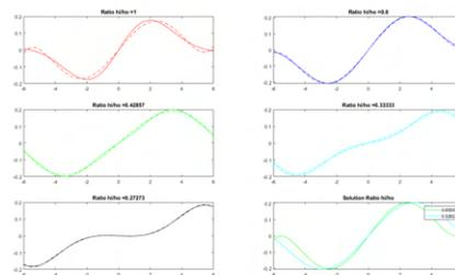
Fig. 2: Forces dependent on relative position of levitator magnet for different ratios.
