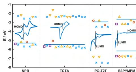
Fig. 1: Exemplary cyclic voltammetry measurements of the various OLED materials and comparison of measured HOMO/LUMO (lines) energies with literature data (markers).
