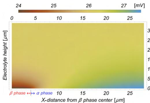
Fig. 2: Potential field in electrolyte domain. Model is implemented in Mathematica.
