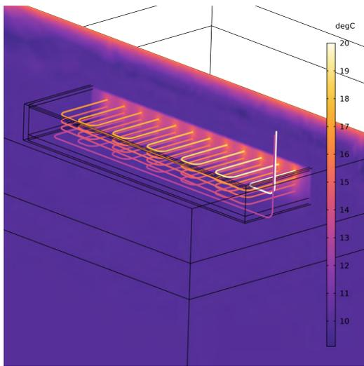
Fig. 1: Thermally activated ground with a downward-opening insulation jacket of 24 cm thickness. The top part of the soil, warmed by the sun, is visible. The temperature of the sand within the insulation is raised by the installed PE pipes, making it capable of storing energy. The glycol-water liquid enters heated into the topmost layer of heating pipes and flows along the pipes down the tank.
