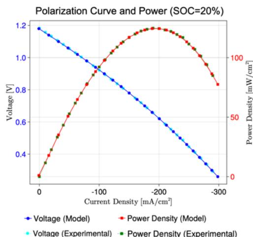
Fig. 2: Cell voltage and power density of a lab sized cell at state of charge 20%.
