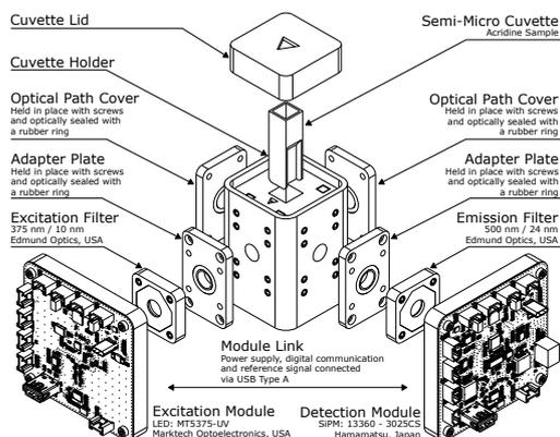
Fig. 1. Possible device architecture that can be used to characterize liquid samples in a semimicrocuvette.
