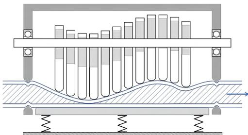
Fig. 1: Cross-sectional view of an exemplary peristaltic pump with a horizontal arrangement of vertically moving sliders that cyclically deform the tube.
