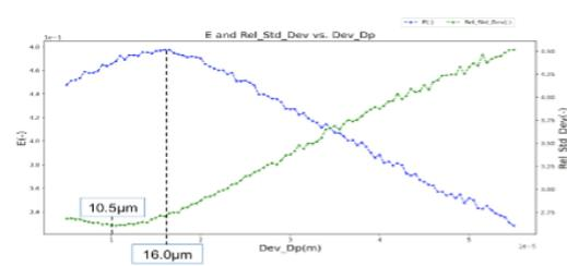
Fig. 3: Coating efficiency (E, blue) and relative Standard batch-based coating deviation (Rel\_Std\_Dev, green) against Standard deviation of particle diameters (Dev\_Dp).
