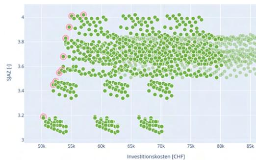
Illustration of a large number of simulations with a financial dimension on the horizontal axis and an ecological dimension on the vertical axis. Each green dot shows the result of one simulation. The simulations marked in orange show the boundary line at which maximum ecological benefit is achieved with minimum financial outlay.
