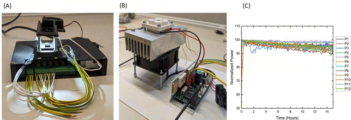
Fig. 1: (A) Aging setup with Maximum power point tracker running under one sun illumination. (B) The Temperature controllable stage which can be paired to the maximum power point tracker and illumination unit. (C) Stability data of some perovskite cells which were fabricated in our lab.
