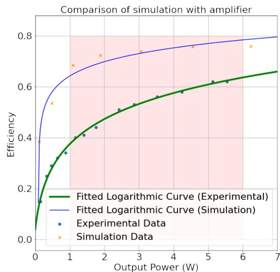
Fig. 2: Comparison between simulation and measurements on the implemented amplifier shows lower measured efficiency than simulated. Key reasons for this discrepancy include unaccounted losses from the DC-DC converter and the use of a suboptimal transformer core that increases losses.
