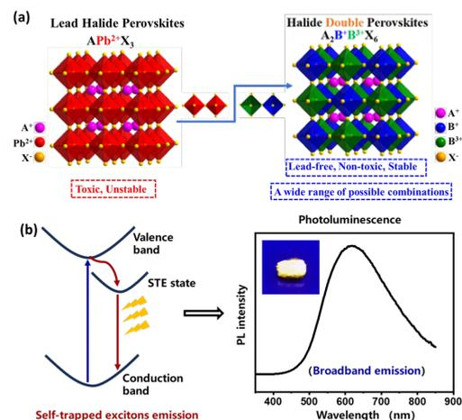
Fig. 1: (a) Schematic view of  $B^+/B^{3+}$  cation substitution from lead halide perovskites ( $APbX_3$ ) to double perovskites ( $A_2B+B_3+X_6$ ). (b) Schematic of the energy level structure and mechanism of STE emission. The PL spectra and optical image are one example of STE emission in lead-free perovskite.
