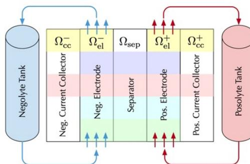
Fig. 1: Simplified model geometry of a flow cell.
