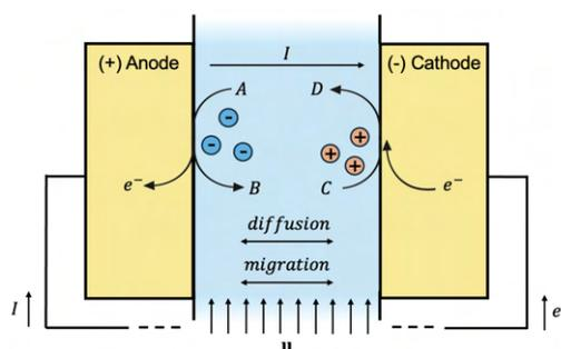
Fig. 1: Schematic of electrochemical flow cell.
