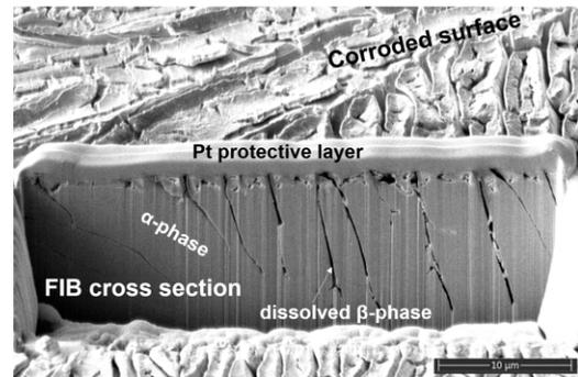
Fig. 1: Surface and cross section of a corroded Ti6Al4V sample exposed to a PBS solution with 3 % hydrogen peroxide for 5 days. The cross section is milled using a focused ion beam (FIB).
