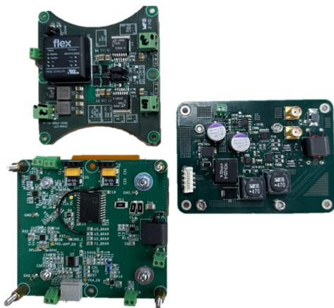
Fig. 1: Image of the circuit boards of the amplifiers: the old ones on the left and the new one on the right.
