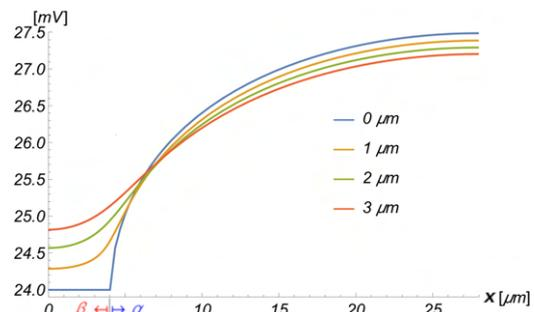
Fig. 3: Potential at different heights in electrolyte.
