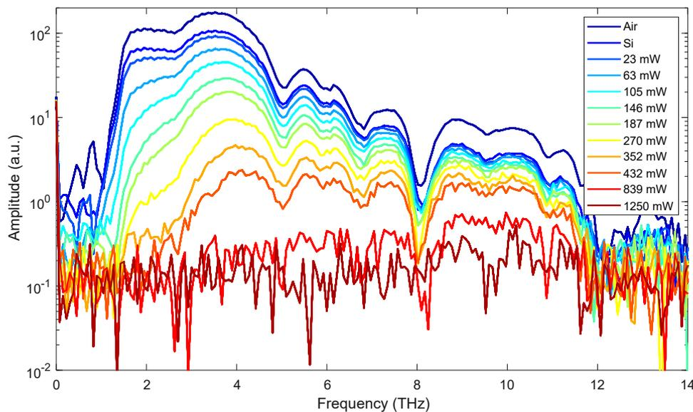
Fig. 1: Different spectra measured on the same silicon sample at different excitation laser powers. The spectrum amplitude decreases with increasing power over the whole measured frequency range. At the highest excitation power, the amplitude was practically zero. Therefore, this silicon in combination with the laser diode could be used as an efficient optical THz modulator with a modulation depth of almost 100 % at the highest optical power.
