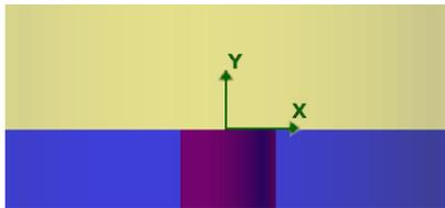
Fig. 1: Schematic of titanium alloy (Ti6Al4V) phases:  $\beta$  (red),  $\alpha$  (blue) under electrolyte (yellow).
