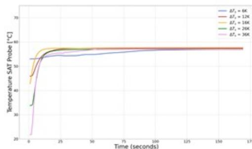
Fig. 2: Temperature curves of the nucleation tests with different subcooling temperatures of the SAT samples.
