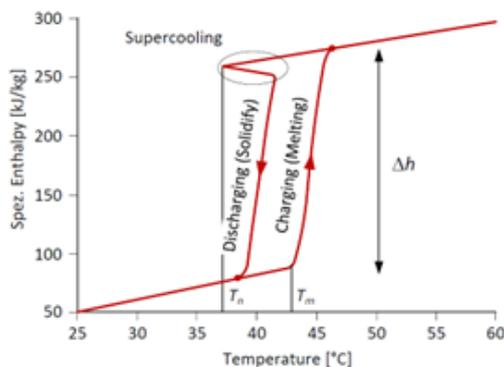
Fig. 1: Enthalpy vs. temperature diagram with melting and solidification hysteresis.
