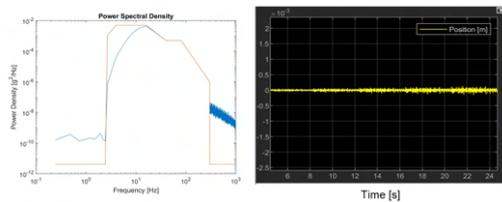
Fig. 1: Illustration of the problem Case 1: In the case of a high bandwidth for the position controller, low frequencies of the desired vibration profile are strongly damped. The graph on the left shows the target profile in red and the simulated profile after 100s in blue. The criteria for position stability ( $|x| < 0.1m$ ) are met (graph on the right).
