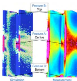
Fig. 1: Simulation based prediction (left) vs. experimentally derived (right) coating pattern of a powder coated U-profile.
