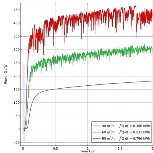
Fig. 2: Power and energy evaluated at the outlet. The laminar nature of the flow is evident at the lowest flow rate, shown by the blue curve. The more turbulent flow at the highest flow rate, red curve, corresponds to the flow shown in Fig. 1.
