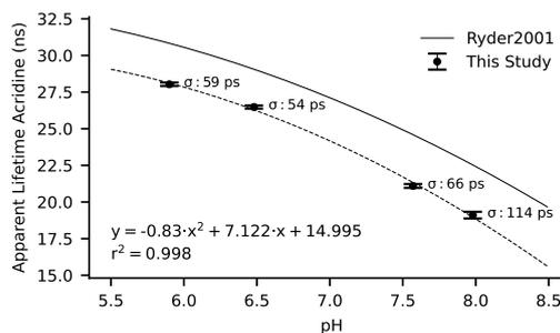
Fig. 2. Measurements of apparent lifetime of at different pH. The samples consist of 1 ml of 0.1 M aqueous K-phosphate buffer at different pH values with an acridine concentration of 0.001 M.
