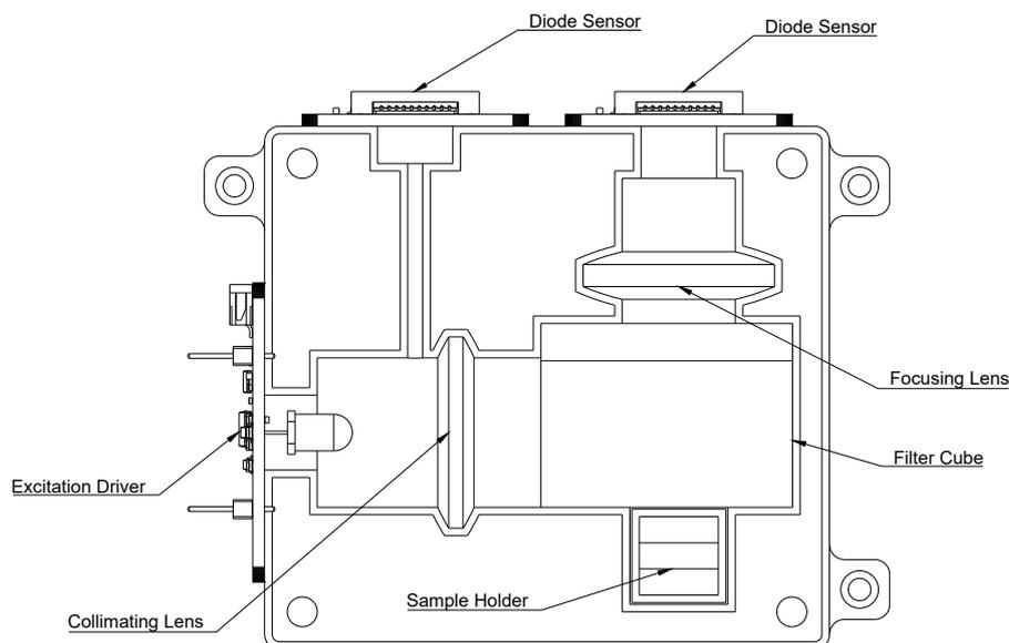
Fig. 1. Sensor module, showing the optical path of the sensor.
