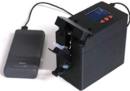
Fig. 1: Final prototype of the point-of-care testing device for the quantification and monitoring of blood ammonia levels using the assay developed by Versantis.
