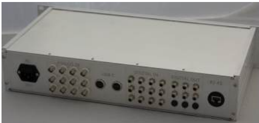
Fig. 1: Prototype of the Digital Wolfram logger in its rugged metallic housing.
