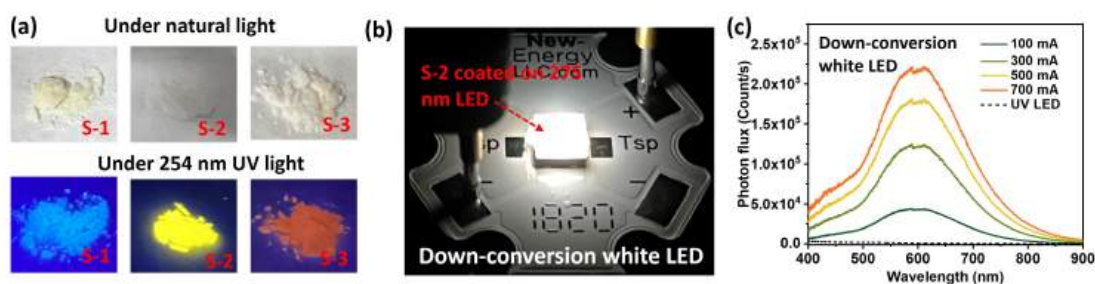
Fig. 1: a) Optical images of three lead-free perovskite derivatives under natural light and 254 nm UV light. b) Down conversion white LED based on S-2 material coated on a 275 nm LED. c) Current-dependent emission of the down-conversion white LED.
