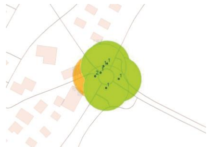
Accumulation of occurred accidents, which have to be analyzed in the Black Spot Management.
