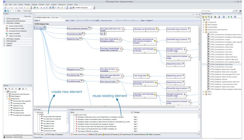
SAHRA allows to capture STPA Step 1 and 2 analysis in the visual style of mind map diagrams. The analysis information is captured by individual elements reflecting for example Keywords, UCAs, Hazards, and Losses. This provides maximum flexibility to the analyst in terms of documenting the analysis. Drag and drop from the lower left panel allows to easily create new elements. Drag and drop from the lower right panel allows to reuse existing elements while inheriting existing relationships.
