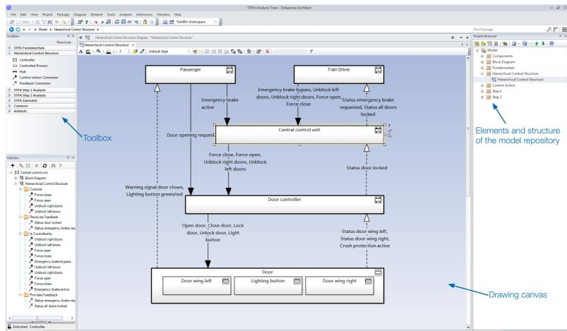
Screenshot of SAHRA as extension for the UML/SysML tool Enterprise Architect. The model of a Hierarchical Control Structure is shown in the center of the screenshot. The controller 'Central control unit' is currently selected. The toolbox (top left) contains all elements needed for capturing STPA diagrams. The model repository and its structure is shown in the repository tree (right).
