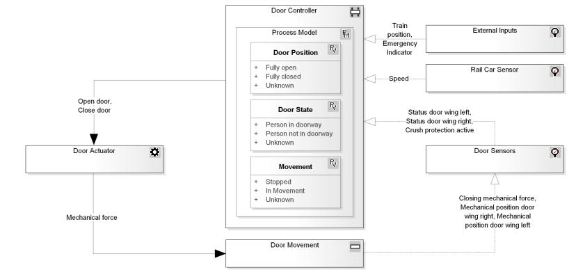
STPA step 2 control loops can be captured just as hierarchical control structures.
