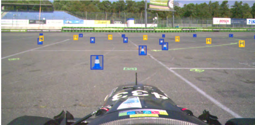
Figure 10.: Object detection example with cones used in formula student races 1
