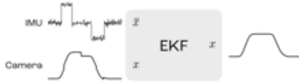
Figure 7: Graphical representation of the working principle of an extended Kalman filter (EKF). Through sensor fusion, a noisy but consistent IMU signal can be combined with a low-noise but inconsistent camera position signal to form a consistent low-noise position measurement.
