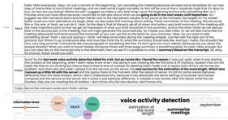
Figure 3.3: Visualization design in the second iteration. A bubble chart shows individual speaker contributions and a clickable word cloud.
