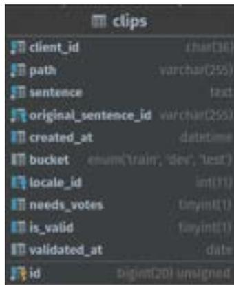
The image shows a screenshot of a database schema for a table named 'clips'. The table has the following columns and data types:
