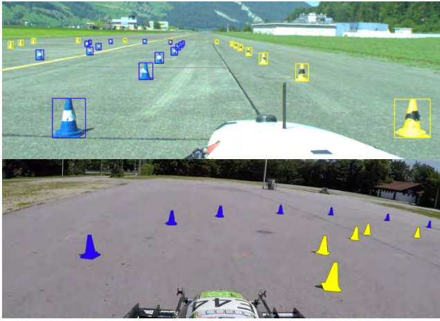
Fig. 7. Two images from the FSO CO Dataset [26]. The upper one shows the ground truth bounding boxes and the lower one the segmentations of those cones.
