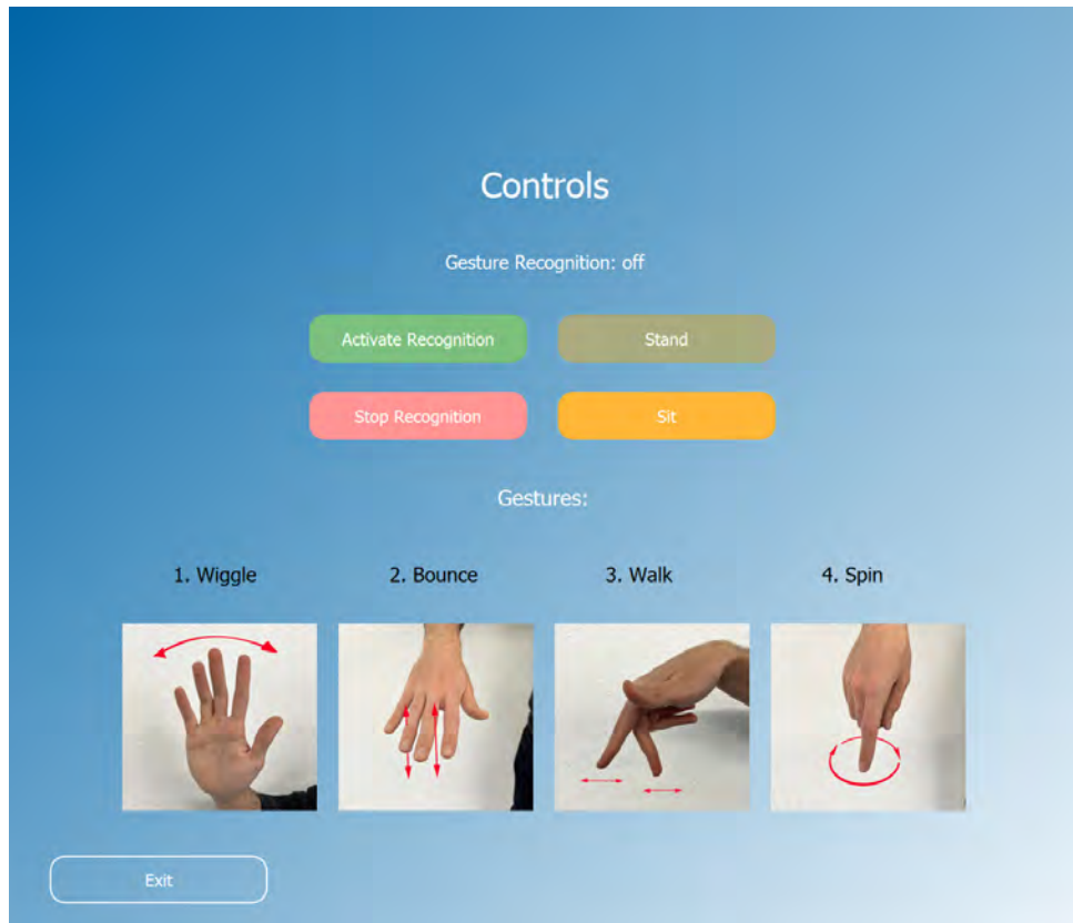
FIGURE 3.8: The UI allows the user to toggle sitting position and gesture recognition.
