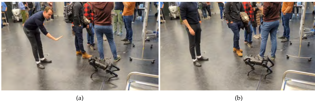
FIGURE 4.1: (a) Participant performing a wave gesture towards the robot, (b) robot leaning from side to side as a response.
