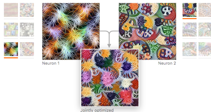
Figure 3.9: By jointly optimising two neurons we can get a sense of how they interact. Reprinted from [4]
