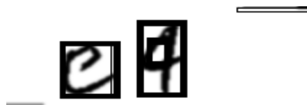
Figure 39 All remaining MSER boxes after applying the minimum and maximum area thresholds to the image.
