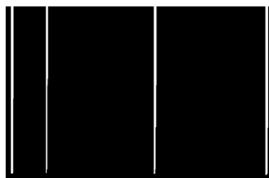
Figure 24 The table lines left after a single erosion and dilation with a large kernel.
