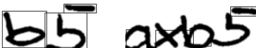
Figure 43 MSER region detection is applied to both images. The left image contains separated parts of a character and the right image contains characters that overlap with each other.
