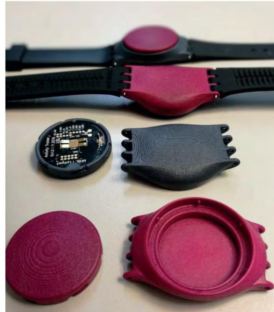
*Figure: Actimeter prototype.*
