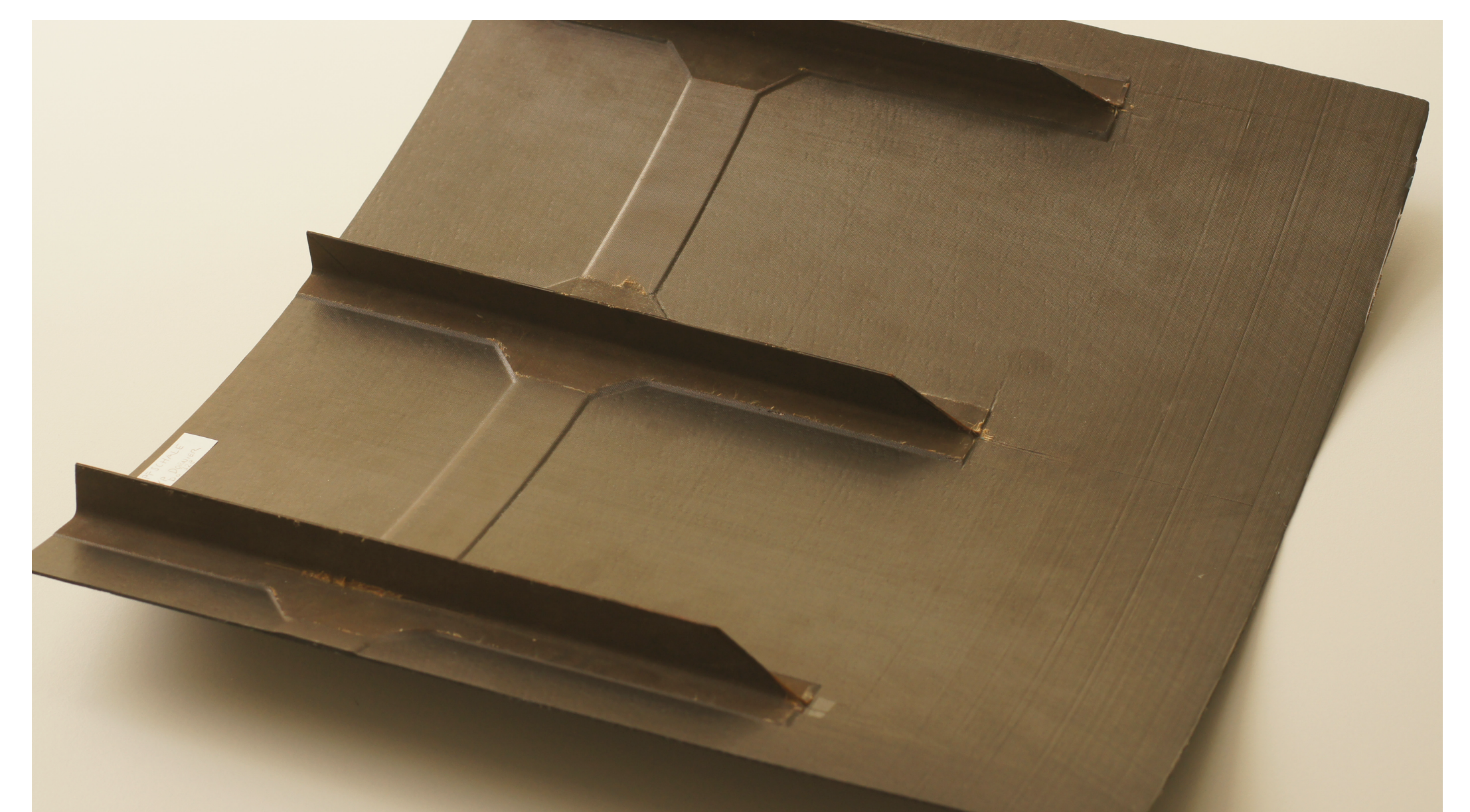
CFRP fuselage with integrated stringers
